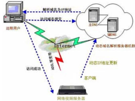
The DDNS process flow diagram of INC-M20xx
